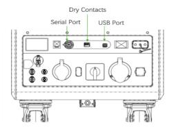
On the back panel there exist the communication ports for different usages.
